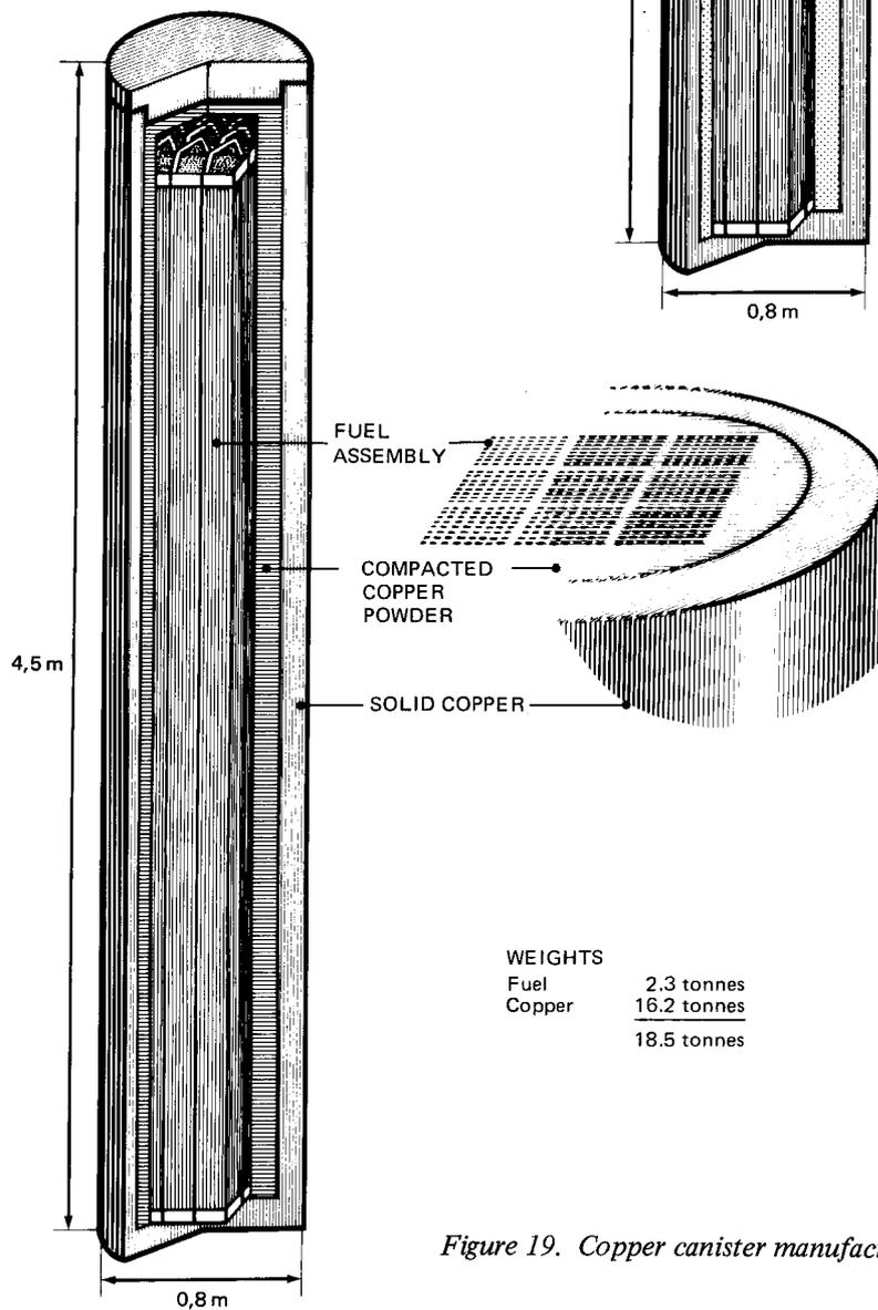
Figure 19. Copper canister manufactured by hot isostatic pressing.
