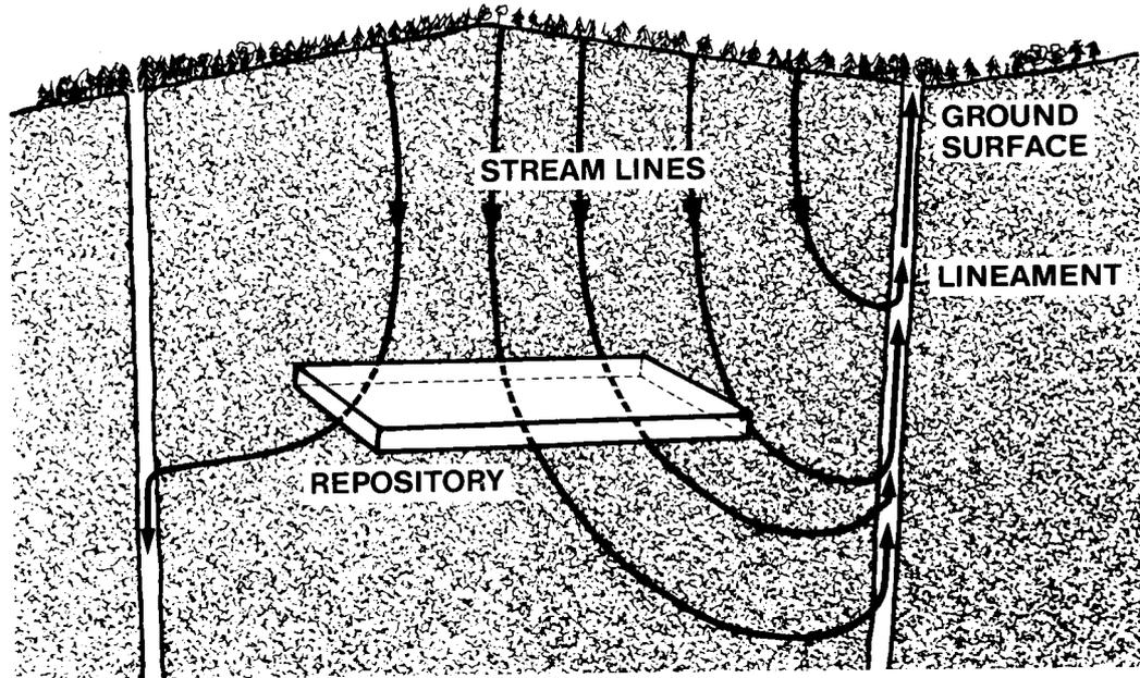
Figure 21. Schematic illustration of groundwater flow.
