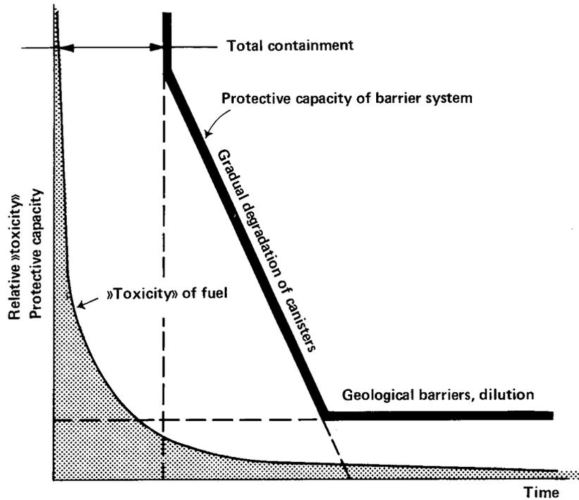
Figure 3. Schematic function of the barrier system.
