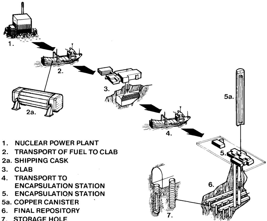
*Figure 2. Handling sequence for spent nuclear fuel.*
