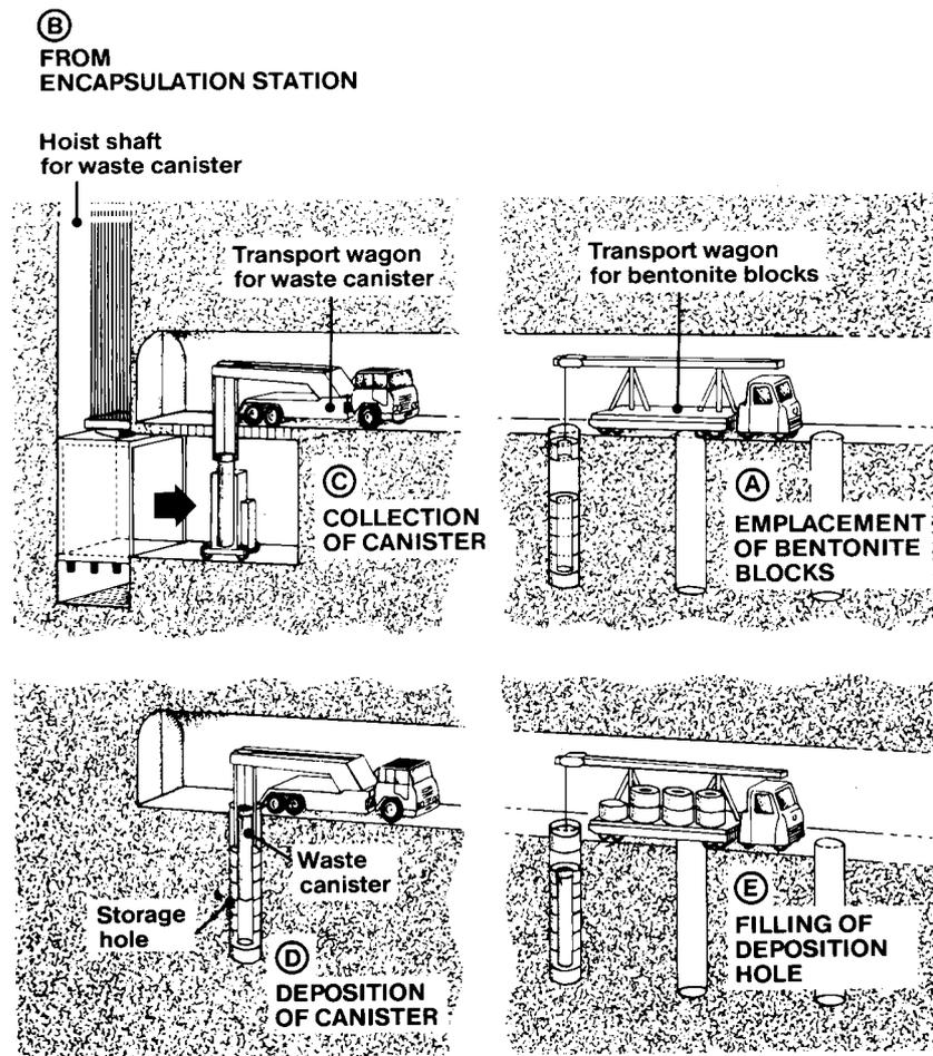
Figure 10. Canister deposition in final repository.
