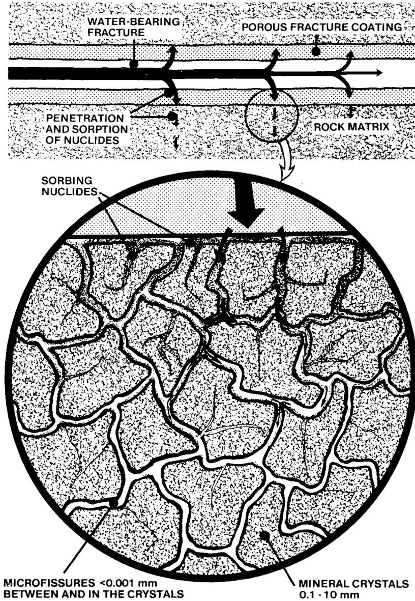
Figure 22. Schematic illustration of sorption and penetration of the radionuclides in the micro-fissures in the rock.
