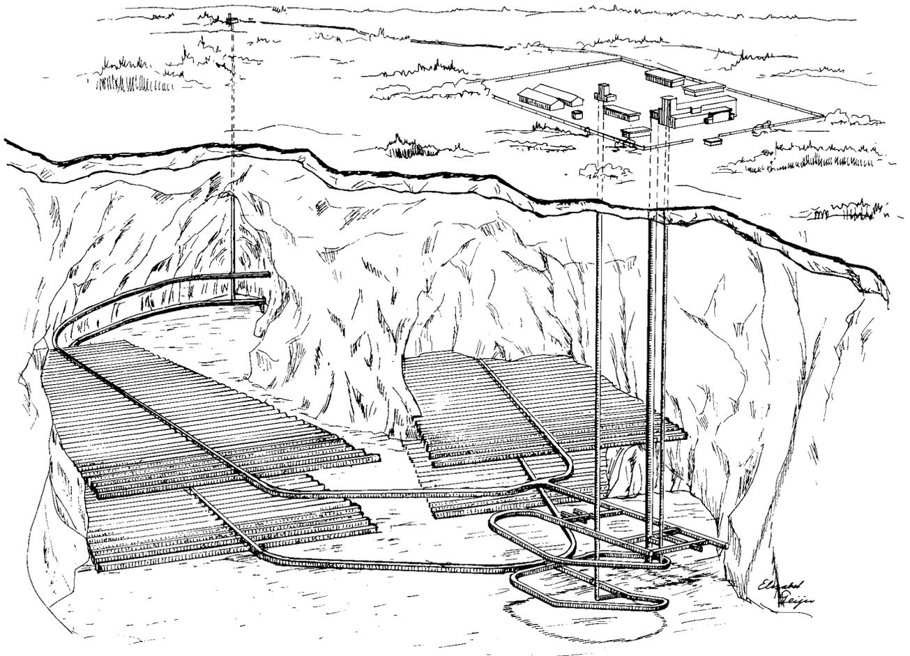
Figure 9. Perspective drawing of final repository.
