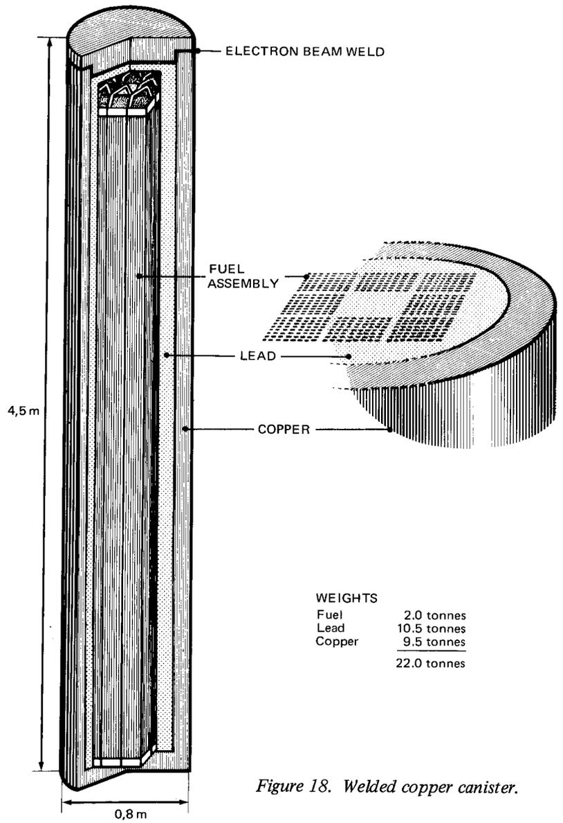
Figure 18. Welded copper canister.
