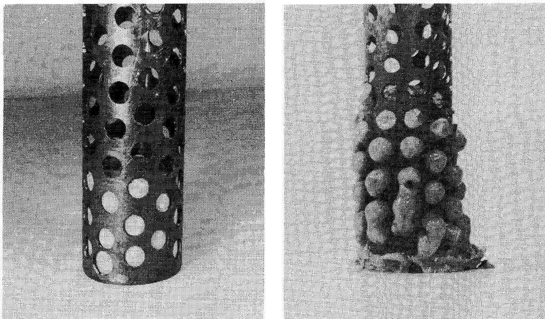
Figure 16. Perforated tube with pressed bentonite pellets for sealing of boreholes.
